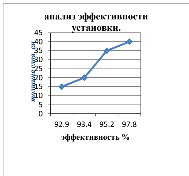
Fig.4. The efficiency of the installation depending on the thickness of the layers.
