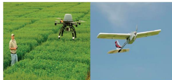
Figure 2: Two types of Drones, Rotary copter (left) and fixed-wing airplane (right) Source: (Strehr 2015)
