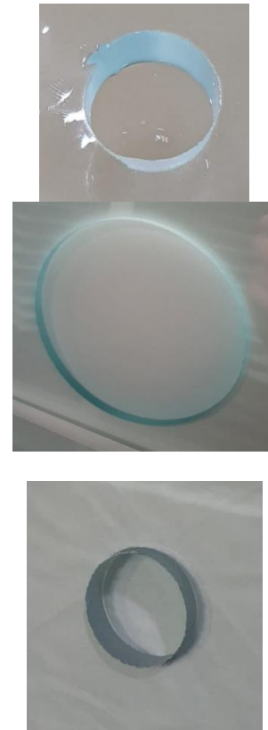
Figure 4.2 Experimental results of the cuts made with inappropriate and appropriate parameters respectively
