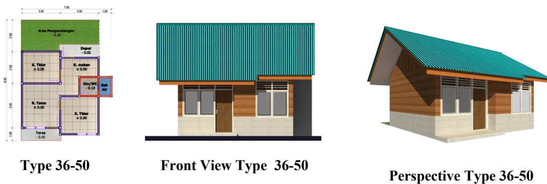
Figure 7. Plans and looks and perspective on the development of type 36 to type 50.
