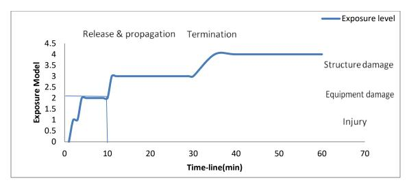
Figure 6: The outcomes of exposure model for a blasting wave of CNG cylinder
