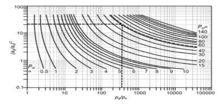
Appendix A-1: Determination of overpressure by the squared ratio of the speed of sound and the the ratio of the initial pressures
