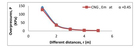
Figure 3: Experimental data on the blast wave [33] and CNG with  $\alpha$  =0.45
