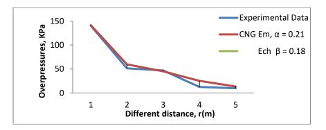
Figure 4: Experimental data on the blast wave and CNG with ( $\alpha = 0.45\&\beta = 0.18$ )
