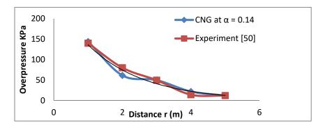
Figure 2: Experimental data and CNG pressure with  $\alpha = 0.14$
