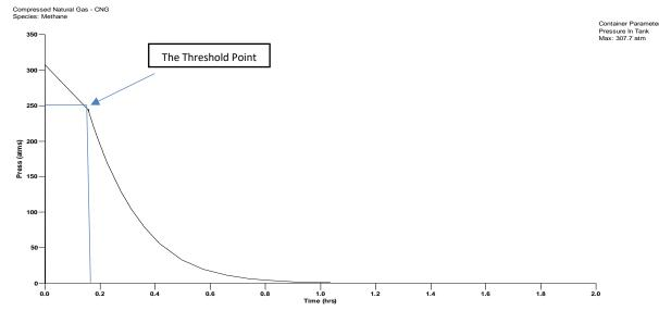
Figure 5: The simulation outcome of resistance time of the CNG cylinder
